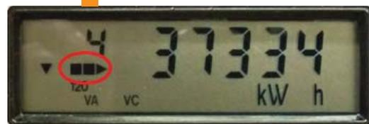
The Commercial Net Energy Meter utilizes left/right arrow indicators and two indicating bars in the middle left section of the display to identify the direction of energy flow. The sequence of this meter matches the residential meter. A left-to-right sequence shows energy is being used by the customer from the electrical system and a right-to-left sequence indicates energy flowing back into the electrical system.
