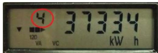
Display code 40 indicates kWh Received. (Energy from customer)
